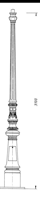
THK-689 Candelabra (one-piece ) with flanged connections Weight: 215 kg
